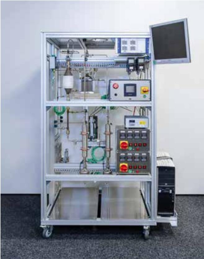
A proprietary catalyst is employed in the first process stage. Long-term testing proved the suitability of the IMM catalyst under harsh temperature operating conditions. Experiments under changing inlet feed-gas composition proved the practical applicability under dynamic regimes of operation.
